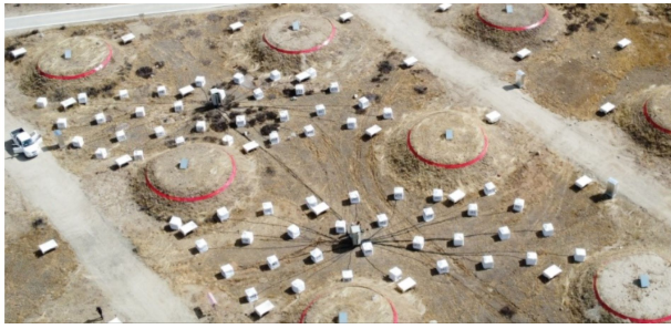
Fig. 1 Photo of the ENDA-64 detector arrays in a bird view.
