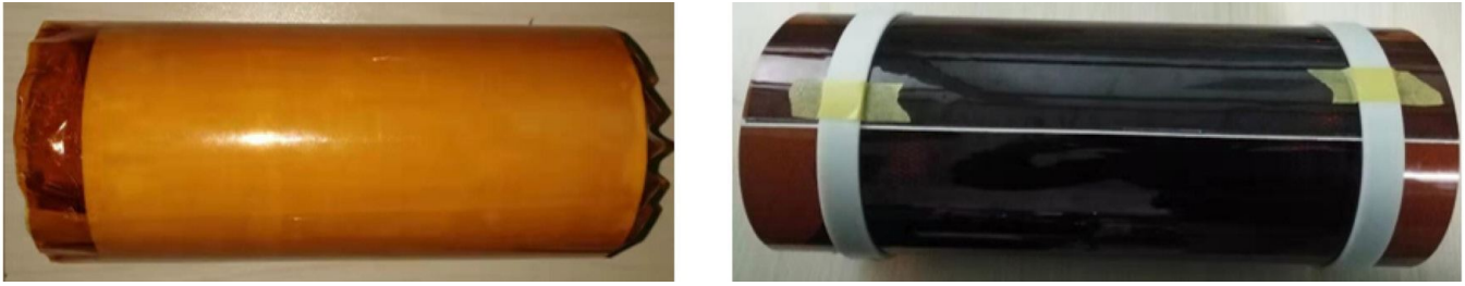
Fig. 3.23 The Rohacell foam-based inner cylinder (left) and aramid honeycomb-based detector model (right) produced in the preresearch stage.
