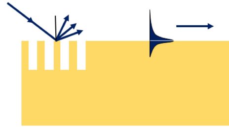
Fig. 5 Schematic of diffraction coupling to SPPs by grating on surface of the metal film.
