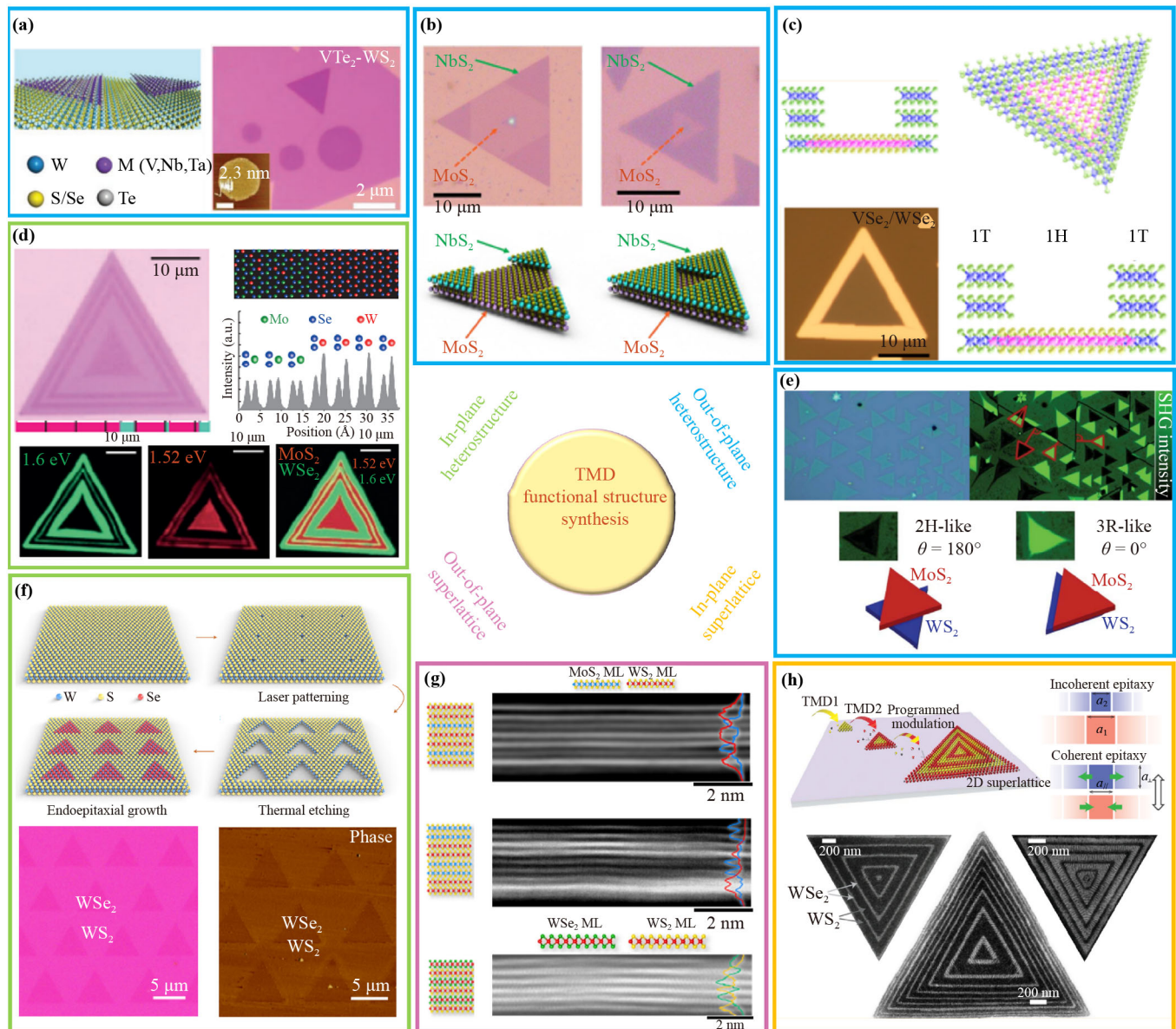
Fig. 5 Synthetic TMD heterostructures. (a) Two-step growth of vertical VTe 2 /WS 2 heterostructures [84]. (b) One-step growth of vertical NbS 2 /MoS 2 heterostructures [85]. (c) Two-step growth of vertical VSe 2 /WSe 2 heterostructures [86]. The second-layer growth initialized at (a) in-plane defects, (b) vertices, and (c) edges, respectively, of the first layers. (d) One-pot synthesis of lateral TMD heterostructures and multi-heterostructures [76]. (e) MoS 2 /WS 2 heterobilayers with tunable stacking orders [87]. (f) Mosaic patterns of lateral TMD heterostructures [77]. (g) Vertical TMD superlattices fabricated by MOCVD [89]. (h) In-plane TMD superlattices grown by modulated MOCVD [90].
