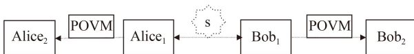
Fig. 2 Shareability of Bell nonlocality under bilateral measurement. Alice_1 and Bob_1 share an initial quantum state with Bell nonlocality via a quantum resource distributor S . They both perform measurements on their own side and send the particles to Alice_2 and Bob_2 , respectively. One identifies the nonlocality sharing between Alice_2 and Bob_2 and so on.
