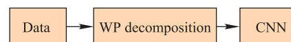
Fig. 3 A flowchart of the proposed scheme. In this flowchart, the “Data” are the data segments in Fig. 1. WP: Wavelet packet; CNN: Convolutional neural network.
