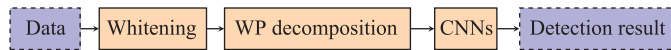
Fig. 1 A flowchart of the proposed scheme. In this flowchart, the “Data” is an observation of time series s(t) , the input into “WP decomposition” is still a time series s_w(t) , and output from “WP decomposition” is a time-frequency map, which is input into the “CNNs”.
