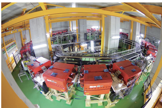
Fig. 7 Photo of Rare-RI Ring (Courtesy of RIKEN) dedicated to mass measurement for exotic nuclei with isochronous mode via individual injection scheme.
