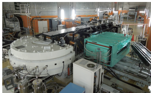
Fig. 8 Picture of SCRIT system which has been developed to measure charge-form factor of exotic nuclei (Courtesy of RIKEN).
