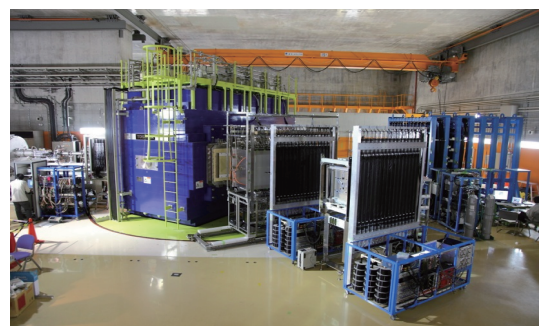
Fig. 5 Photo of SAMURAI spectrometer (Courtesy of RIKEN). A large-gap super-conducting magnet are combined with standard detectors; large size drift chambers, hodoscopes and neutron TOF detector array.
