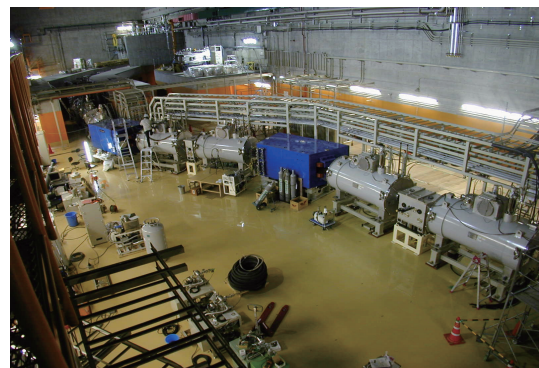
Fig. 3 Photo of a part of BigRIPS in-flight separator (Courtesy of RIKEN). RI beams produced at the first stage of BigRIPS (left, behind the concrete wall) are transmitted to the second stage and the beams identified at the second stage are delivered to experiment sites.
