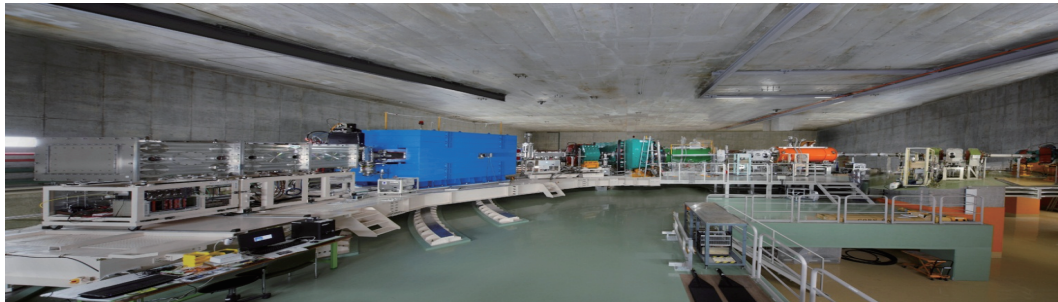
Fig. 6 Photo picture of SHARAQ spectrometer (Courtesy of CNS, Univ. of Tokyo). RI beams through a special beam line designed to achieve a dispersion matching optics mode come from left.
