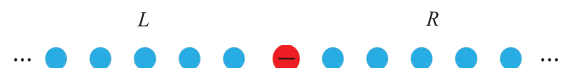
Fig. 11 A schematic plot of a single-level quantum dot coupled to two one-dimensional tight-binding leads.
