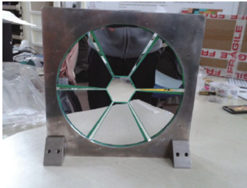
Fig. 6 One annular silicon array.
