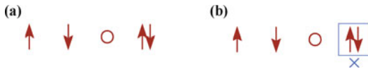
Fig. 3 (a) Four possible electron states at a lattice site; (b) The double occupancy state is forbidden under the Mott constraint (2).
