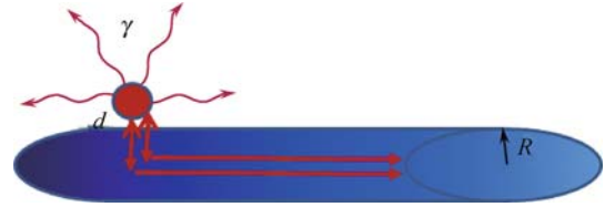
Fig. 1 Schematic illustration of the QD-nanowire system: a QD emitter (red dot), is placed at a distance d of a metallic nanowire (blue cylindrical wire) with radius R .
