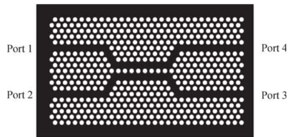
Fig. 25 The schematic diagram of a photonic crystal directional coupler. The signal is input from port 1, and the output signal is detected at port 3, whose intensity sensitively depends on the coupling length in the central region of the device that can be modulated by Kerr nonlinearity.
