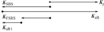
Fig. 31 The wave vector scheme of the experiment, \mathbf{K}_p , \mathbf{K}_{\text{SBS}} , \mathbf{K}_{\text{aB}} , \mathbf{K}_{\text{FSRS}} , and \mathbf{K}_{\text{aR1}} represent the wave vectors of laser, SBS, acoustic phonon, FSRS, and optical phonon, respectively.
