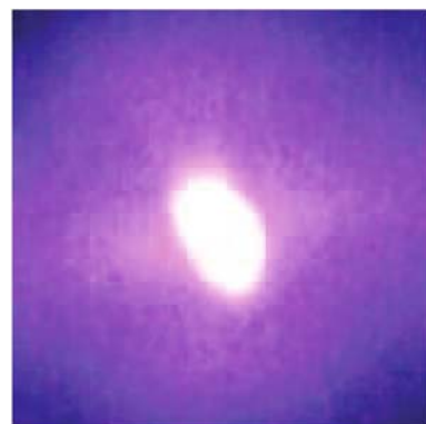
Fig. 4 Image of cold ytterbium ^{174}\text{Yb} atoms in the 399-nm MOT.
