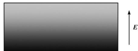
Fig. 5 Sketch showing a graded metallic film with a gradient along z axis perpendicular to the film. The electric field E is parallel to the gradient along z axis.
