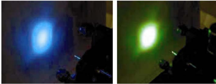
Fig. 13 Output of anti-Stokes line emission in a PCF by pump pulses polarized along ( left ) the fast and ( right ) the slow axis of the fiber core.
