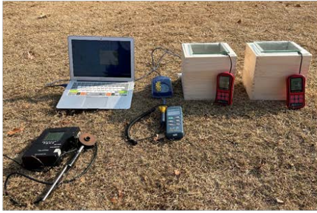
Figure S7 Performance demonstration of the hydrogel-glass in a house model. (a) Photograph on experiment setup. (b) Temperatures of the hydrogel-glass, normal glass and environment.
