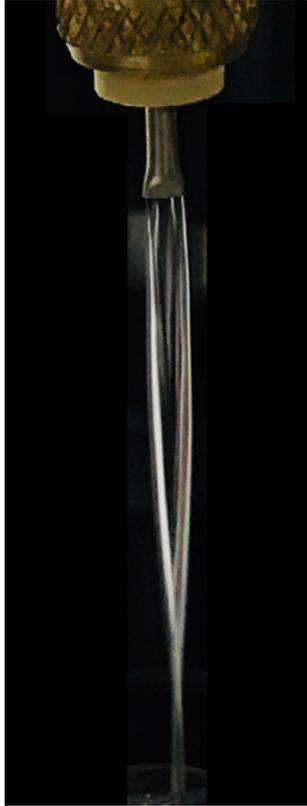
**Fig. 10** Photo of a 120  $\mu\text{m}$  thick water film formed by a water jet with a flat nozzle [62]. The laser beam is focused into the center of the film where is flat and stable
