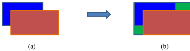
Fig. 5 Box fusion algorithm. (a) Two detection boxes; (b) fused detection box. The background green box is the output box obtained by fusing the two detection boxes in (a)
