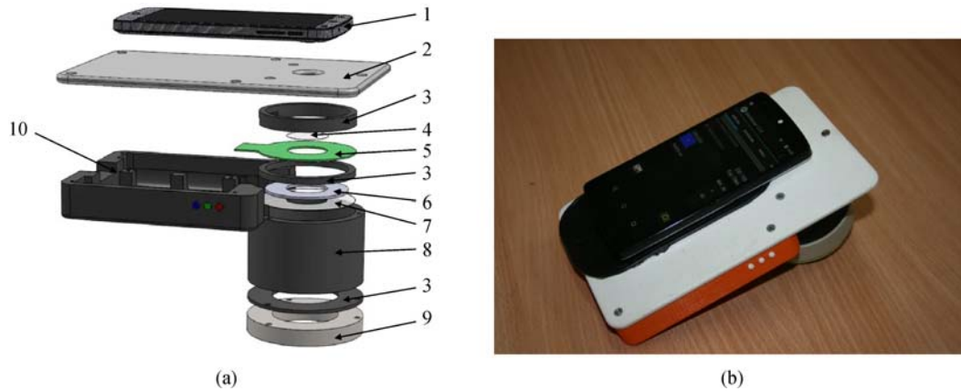
Fig. 2 Design details of the smartphone-LED prototype device (a) and its outlook with a smartphone on it (b). 1 – smartphone, 2 – sticky fixing platform with a camera window, 3 – holding ring, 4 – polarizer of the detected light, 5 – LED ring comprising four sets of LEDs, 6 – light diffuser, 7 – illumination polarizer (oriented orthogonally to the polarizer 4), 8- screening spacer, 9 – silicone skin contact ring, 10 – compartment for batteries and electronic components
