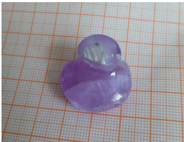
Fig. 1 As-grown \text{Nd}:\text{GdNbO}_4 crystal boule
