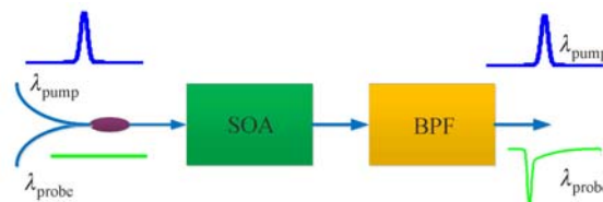
Fig. 5 Pump-probe technique to measure the carrier recovery time
