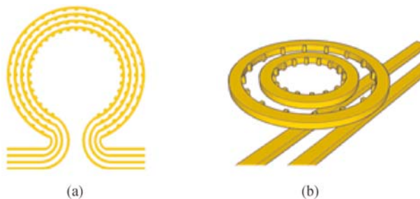
Fig. 8 Sketch of integrated OAM (de-)multiplexer OAM. (a) \Omega -shaped device; (b) concentric ring devices
