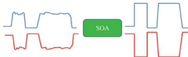
Fig. 9 Illustration for principle of XGC
