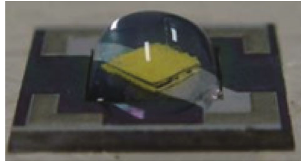
Fig. 7 Singulated component of LED WLP [6]
