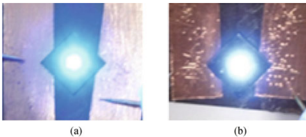
Fig. 14 Illumination of LED WLP prototype with LED flip chips mounted on silicon sub-mount with cavities and TSVs [7]: LED package (a) without phosphor printing; (b) with phosphor printing
