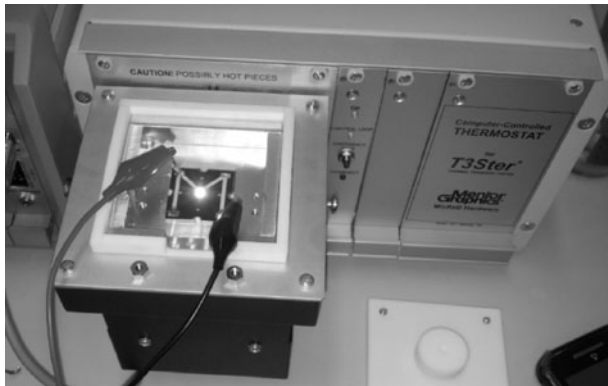
Fig. 3 Photo imaging of test set-up for measuring thermal resistance
