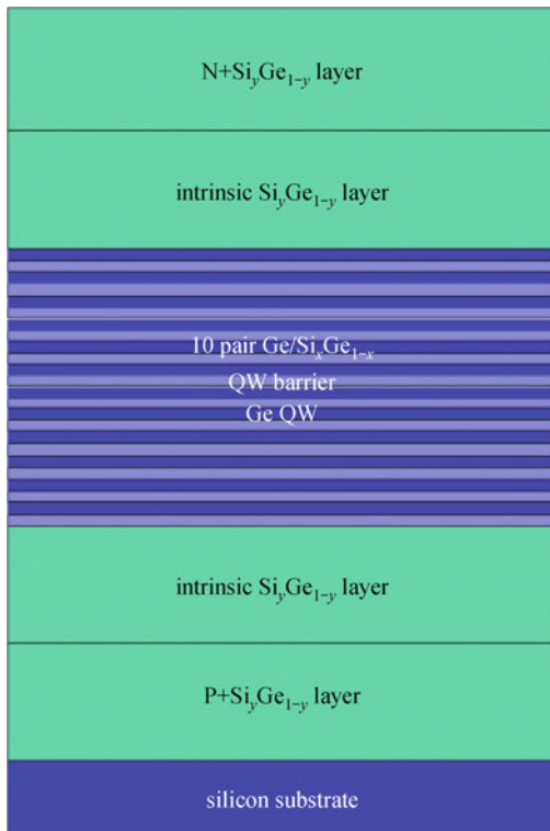
Fig. 1 A p-i-n structure on Si with Ge/ \text{Si}_{1-x}\text{Ge}_x QWs on relaxed \text{Si}_{1-z}\text{Ge}_z buffer
