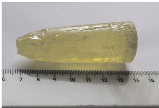
Fig. 1 Photograph of as-grown AGGS boule
