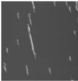
Fig. 5 Quality of 1.7 \mu\text{m} FLC cell alignment (FLC cell is placed between crossed polarizers; micro-photo dimension is 140 \mu\text{m} \times 140 \mu\text{m} )
