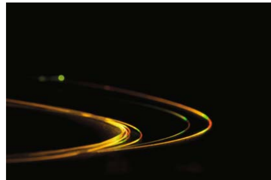
Fig. 6 Green-guiding hollow-core photonic band-gap fiber excited using a broadband supercontinuum source (bright colors visible when the fiber is most close to directly approaching the camera are a result of the dependence of the band-gap edge on angle and wavelength)
