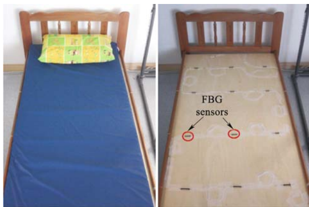
Fig. 2 Sensor array deployment on a bed
