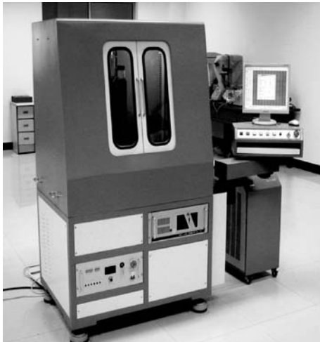
Fig. 3 Laser micro-cladding fabrication system
