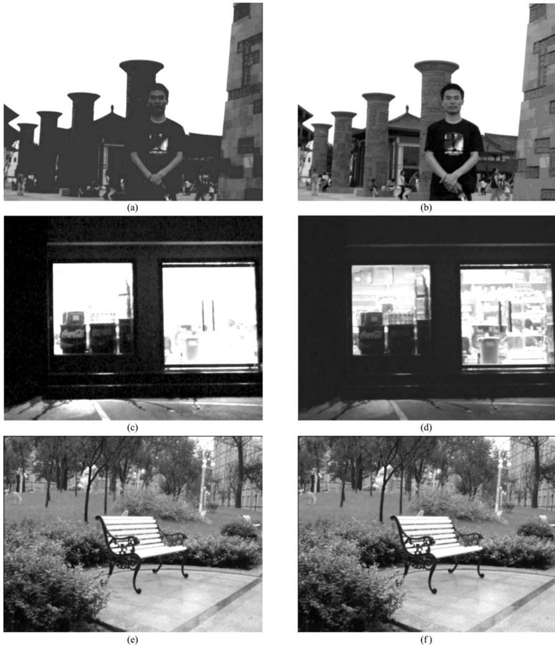
Fig. 7 Experimental results. (a) Backlighting scene; (b) AE result for (a); (c) frontlighting scene; (d) AE result for (c); (e) ordinary scene; (f) AE result for (e)
