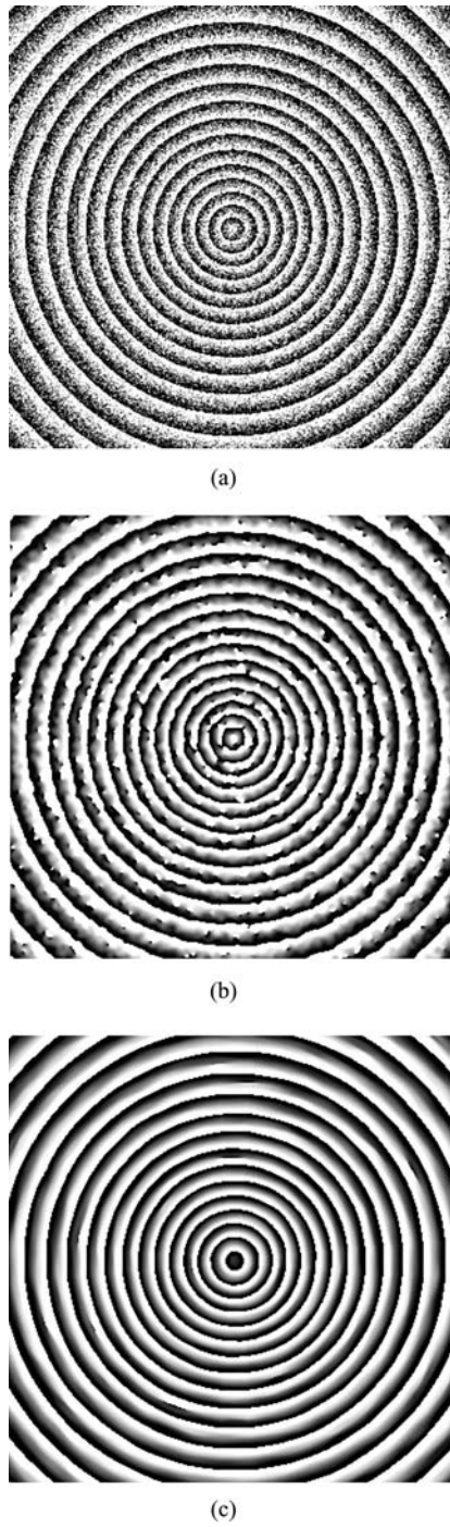
Fig. 6 (a) Simulated saw-tooth phase map; (b) resultant map filtered six times by sine/cosine filter with a window size of 3 \times 3 ; (c) resultant map filtered three times by FCW-SCF with a window size of 3 \times 15
