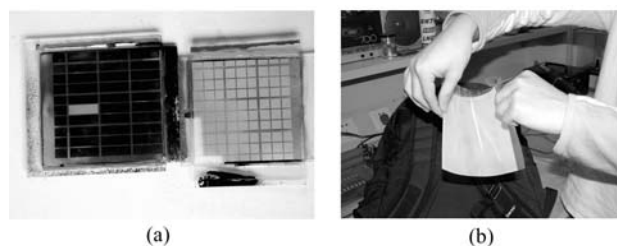
Fig. 5 ZFB-LCD by combination of surface deposited polymer and polymer network. (a) ZFB-LCD in glass substrates; (b) ZFB-LCD in PETs
