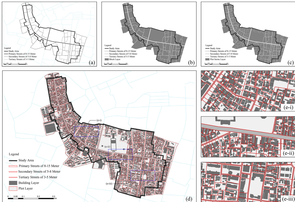
Fig. 6 Study area and morphological hierarchy of Xijie Historic District: (a) street layer; (b) block layer; (c) plot series layer; (d) plot and building layer; (e) details of urban form.
