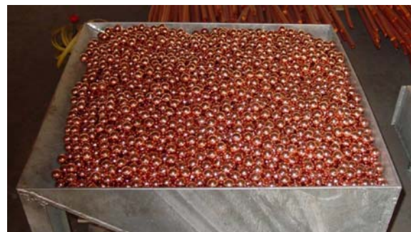
Fig. 11 The phosphorous copper balls formed by SR at room temperature
