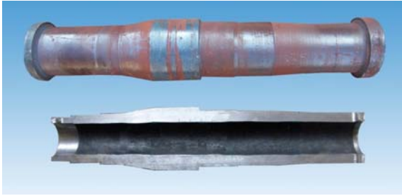
Fig. 12 The hollow axle sleeve formed by CWR
