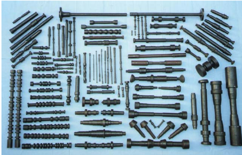
Fig. 7 Some parts produced by CWR
