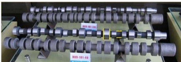
Fig. 10 The precision CWR camshaft blanks and finished products
