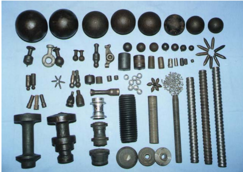
Fig. 8 Some parts formed by SR
