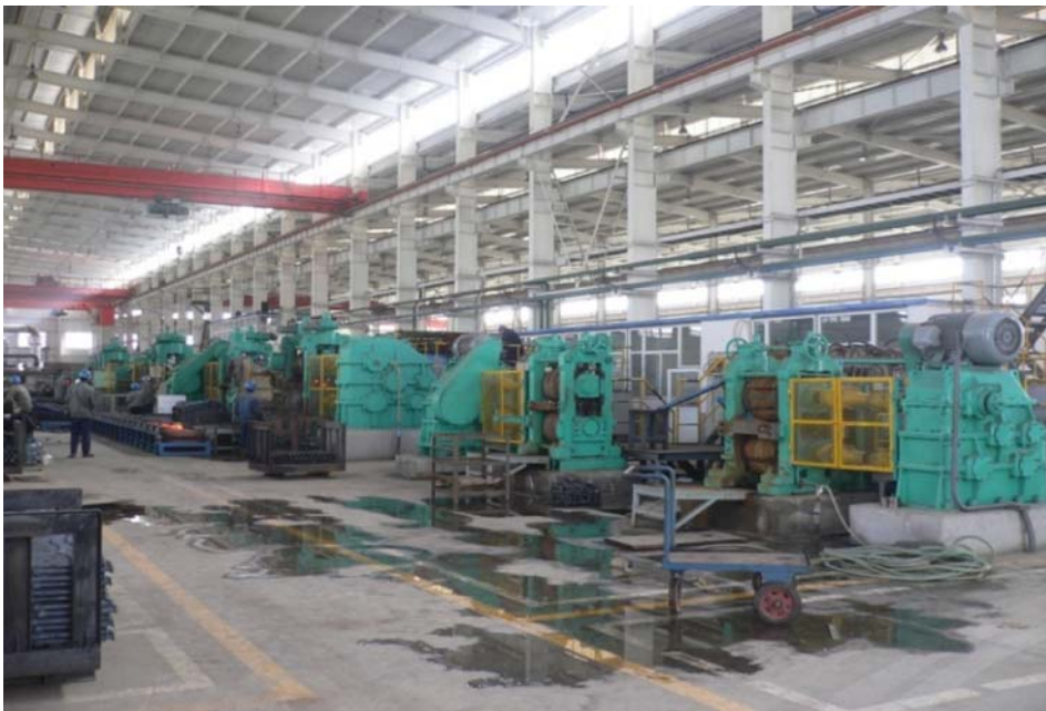
Fig. 5 Professional CWR plant for transmission shafts
