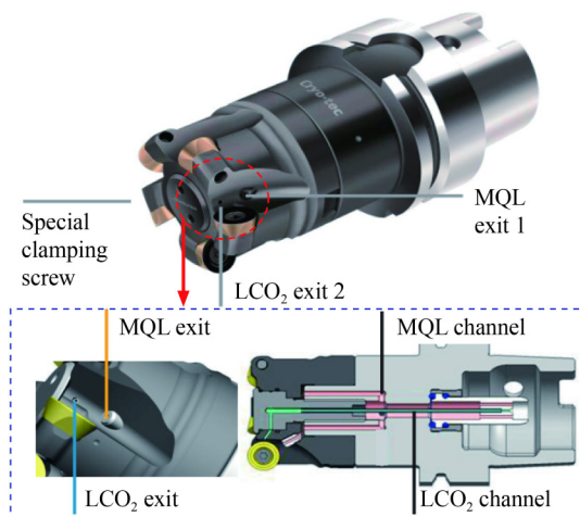
Fig. 13 New Cryo-tec™ milling cutter structure. Reproduced from Ref. [58] with permission from Elsevier.
