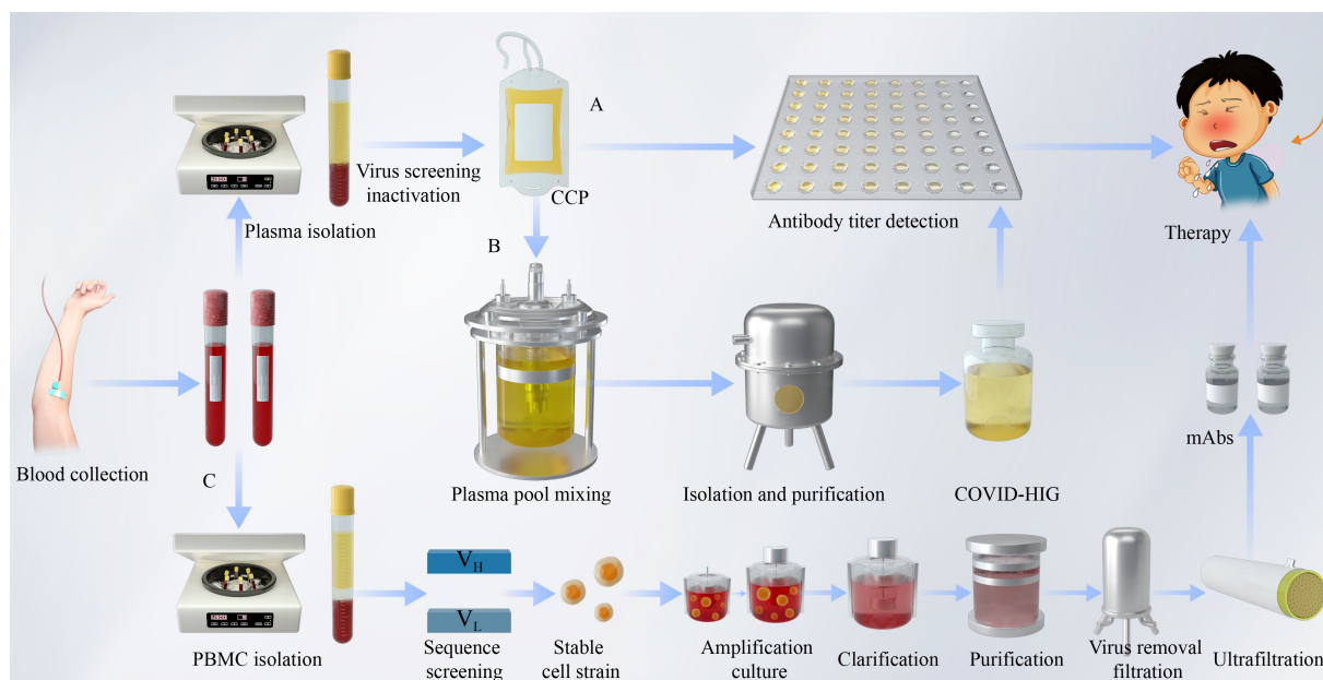
Fig. 2 Schematics of obtaining and industrial production of CCP, COVID-HIG, and mAbs. Blood is collected from a patient who recovered from COVID-19. (A) For CCP preparation, plasma cells are first obtained by centrifugation, and viruses in serum are removed or inactivated. Then, the SARS-CoV-2-specific antibody is detected. Qualified samples can be used for CCP therapy. (B) For COVID-HIG preparation, blood is centrifuged to collect the supernatant plasma, and plasmas from different individuals are mixed, inactivated, separated, and purified. Antibody testing is performed, and qualified samples can be used for COVID-HIG therapy. (C) mAbs are prepared by single B cell sorting technology. First, peripheral blood mononuclear cells (PBMCs) are isolated from the whole blood. Then, target B cells are screened from PBMCs by using flow cytometry. The gene sequence of the SARS-CoV-2 specific antibody secreted from target B cells is analyzed. Plasmid expression of SARS-CoV-2-specific antibody is conducted, and a stable cell line is generated by incorporating the transfection plasmid into the host CHO cell genome. The CHO cells are inoculated with stepwise amplification, and the culture supernatant is clarified by filtration, purified through chromatography, and concentrated through ultrafiltration. After the virus is removed, the mAb formulation is obtained for COVID-19 treatment.
