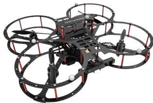
The deployed quadrotor robot: qanser QDrone.
