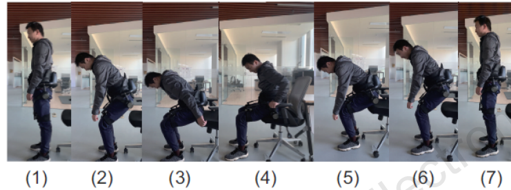
Fig. 17 A sit-to-stand cycle with exoskeleton assistance
