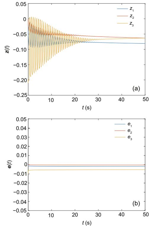
Fig. 4 States  $z(t)$  (a) and errors  $e(t)$  (b) with  $\alpha = 0.21$  and  $\tau = 0.37$
