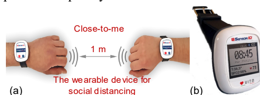
Fig. 16 Graphic representation of the Close-to-me system (a) and front view of the wearer to monitor social distancing (b) (Partitalia, 2020a)
