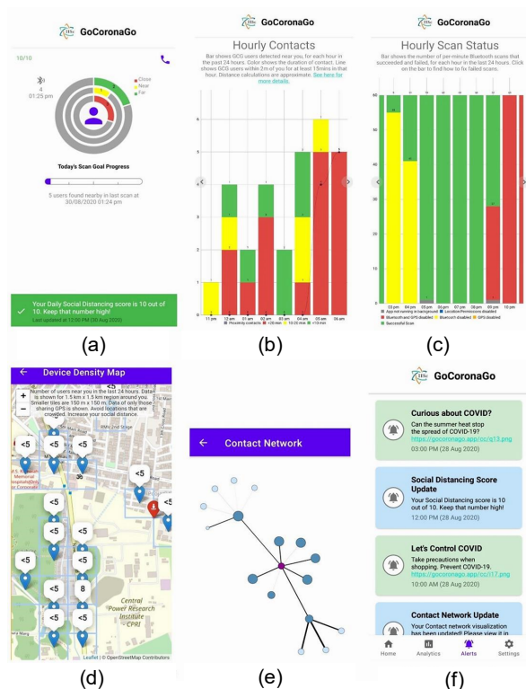
Fig. 24 User interface and analytics in the GCG v0.7 Android App: (a) main screen; (b) hourly contacts; (c) hourly scans; (d) device density heatmap; (e) contact network; (f) alerts panel
