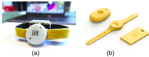
Fig. 18 iFeel-You bracelet developed by the Italian Institute of Technology (Italian Institute of Technology, 2020) (a) and line of wearable products manufactured by Estimote Co. for containing the COVID-19 pandemic (Estimote, 2020) (b)
