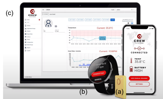
Fig. 8 Overview of the main components included in the CREW system: (a) sensor platform; (b) wearable digital thermometer sensor; (c) cloud platform (8 West, 2020)
