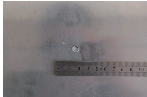
Fig. 4 The penetrated hole on the front bumper (the size is 170 mm × 114 mm)
