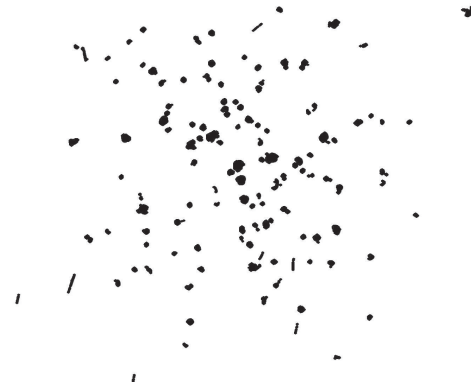
Fig. 14 All craters in the image of the rear wall (the size is 2000 mm × 2000 mm)
