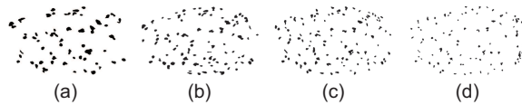
Fig. 7 Key fragments of debris clouds after pre-processing (the size is 80 mm × 53 mm). In (a)–(d), the number of fragments is 60, 90, 109, and 90, respectively
