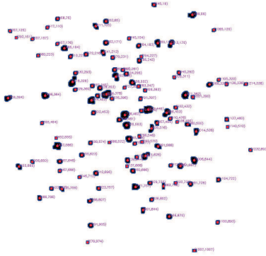
Fig. 16 Centroids of contours of craters in Fig. 15 (the size is 2000 mm × 2000 mm)
