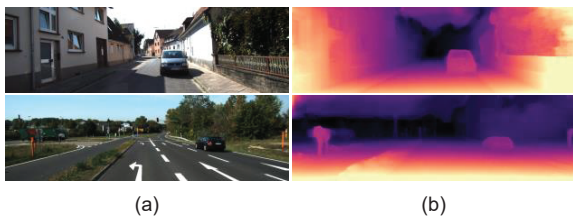
Fig. 1 Our depth prediction results on the KITTI dataset using Eigen split: (a) original images; (b) depth maps predicted by our models
