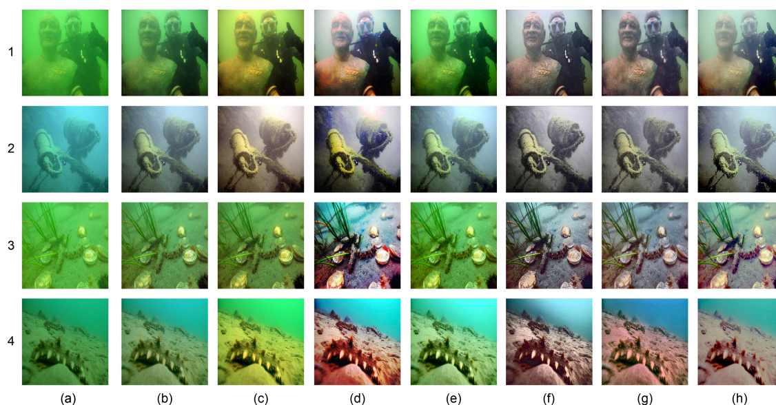
Fig. 9 Comparison of underwater image enhancement methods: (a) underwater raw images; (b–h) images obtained using Iqbal et al. (2007), Iqbal et al. (2010), Ghani and Isa (2014), Huang DM et al. (2018), Pan et al. (2018), Fu et al. (2014), and Zhou et al. (2019b)'s methods, respectively
