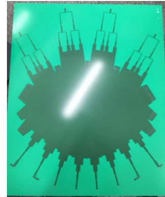
Fig. 9 Fabricated Rotman lens with power dividers
