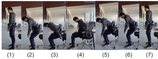
Fig. 17 A sit-to-stand cycle with exoskeleton assistance
