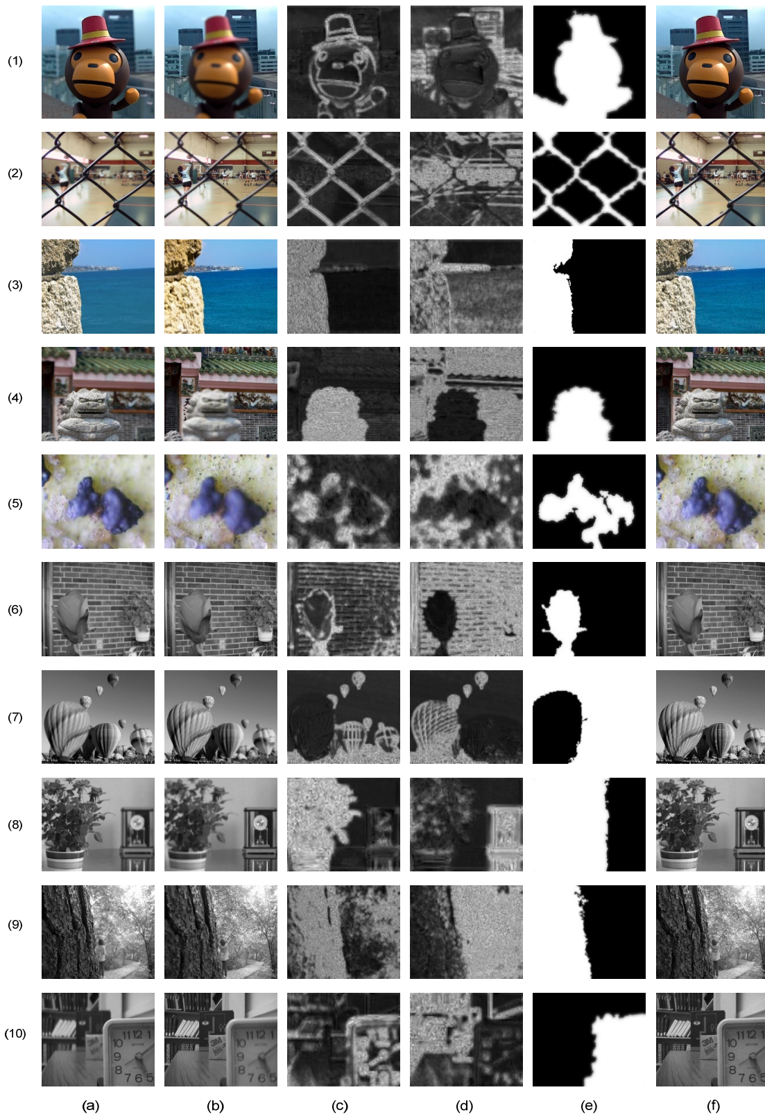
Fig. 3 Ten sets of examples: (a) source image A ; (b) source image B ; (c) score map S_A ; (d) score map S_B ; (e) decision map D_s ; (f) fused image F
